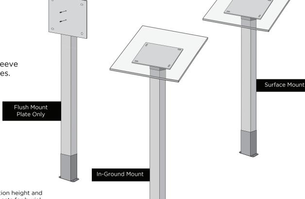
\* Post length is determined by panel height, installation height and burial depth. Panels over 24" h may require longer posts for burial
